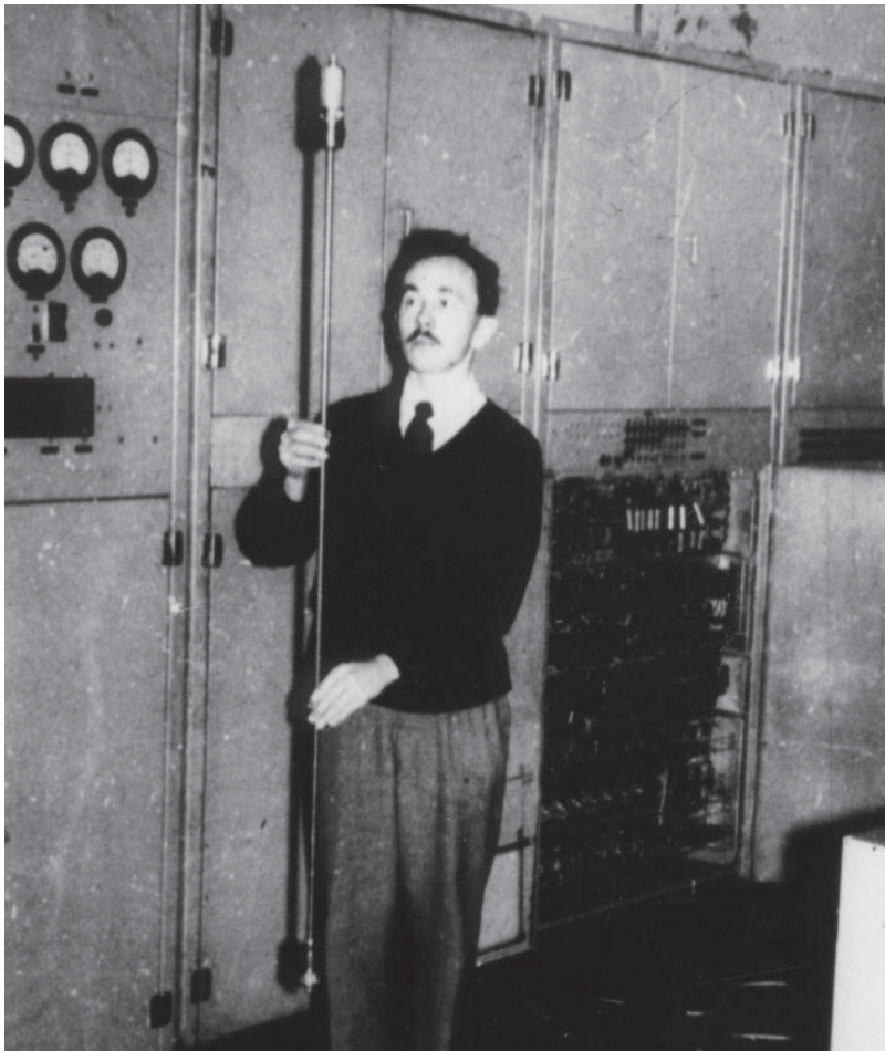
Jurij Semkiw displaying a mercury delay line. 1956.
