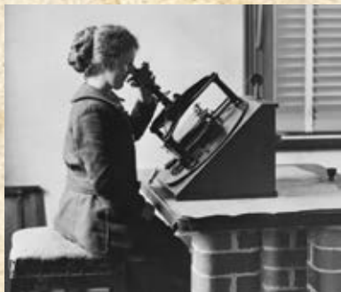
Women as Computer. Female assistant using a photographic plate measuring machine to measure the precise positions of stars for the international Astrograph Project, c1905. Source: Museum Victoria.
