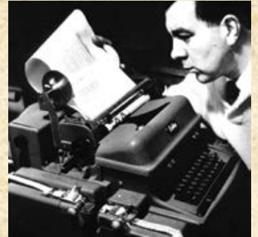
John Russell at the Flexowriter, reading output from CSIRAC, c1959. Image courtesy CSIRO.
