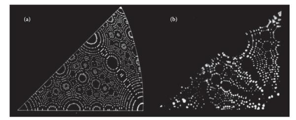
Figure 2. A CSIRAC computer simulated pattern for a face centered cubic crystal (a). compared with the corresponding area of a field ion micrograph of tungsten (b). then be written in a language similar to earlier forms of BASIC. CSIRAC was no longer a mystery and we could calculate the positions of all the atoms on the surface of a spherical metal crystal.
