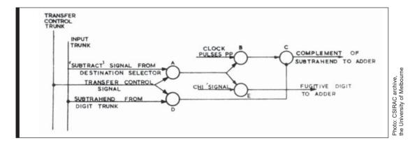
Circuit diagram of the Complementor. that the computer be transferred to the Aeronautical Research Laboratories in Melbourne but later it was decided that it should be housed where it was more readily accessible to different users.
