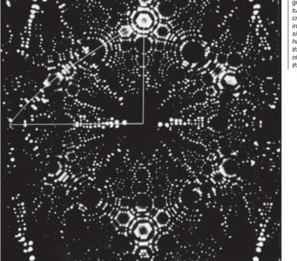
Figure 1. A field ion micrograph of a very sharp tip of tungsten, a body centered crystal. The white spots indicate the positions of single atoms. The image has the same symmetry as the crystal and is made up of repeated reflections of the marked triangular area.
