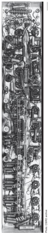
A section of the CSIRAC circuitry – time selector.
