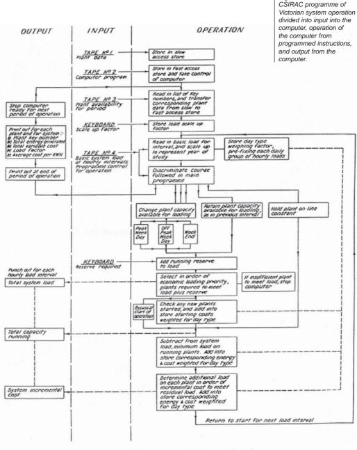
Flow Diagram of Computer Operation.
