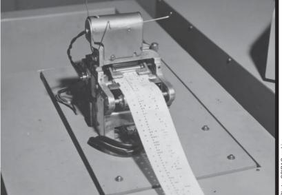
12-hole paper tape reader used for loading programs (and data) into CSIRAC's memory. c.1956.
