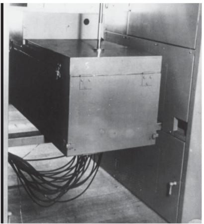
1940's memory technology. CSIRAC's mercury delay line temperature controlled cabinet with thermometer on top. c.1956.
