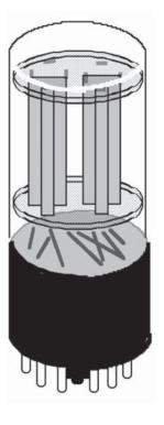
Diagram of a 6SN7 valve and the connections for the valve The Mk 1 used about 2,000 valves. Many of these were 6SN7 twin triodes so this represents under 4,000 logic elements. It was a very economical design. The machine was composed of a considerable number of circuits similar in style to this:
