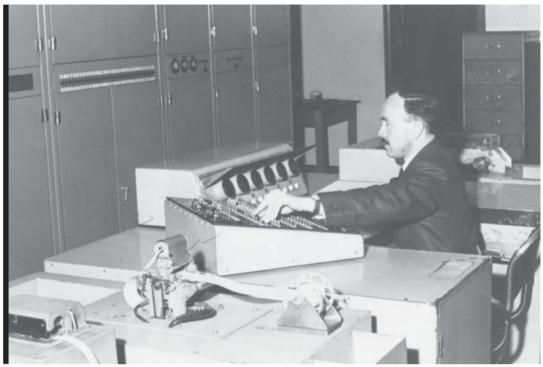
A view of Jurij Semkiw at operating console, with 12-hole tape reader in background and 5-hole tape reader in foreground. Main computer in the background at left. Taken in the early 1960s. and continued operation. If, for example, it was found that the memory was losing bits, users were permitted to boost up the voltage.
