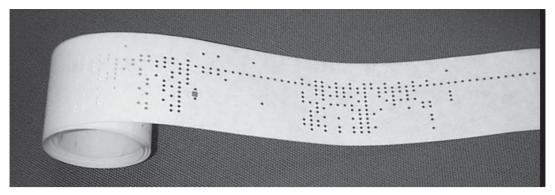
First generation programmers had to design their programs then use the special purpose hand punch to prepare a paper tape containing binary instruc- | 12-Hole paper tape tions. Later, they could also use a library of subroutines to do particular jobs such as maths functions and formatted output. In Melbourne, these subroutines lived four to each small box in a wooden rack near the computer. An "editing station" allowed the required library tapes to be copied onto the main program tape.
